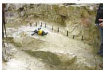
Extracting block of sandstone using traditional methods. Swinton Quarry
